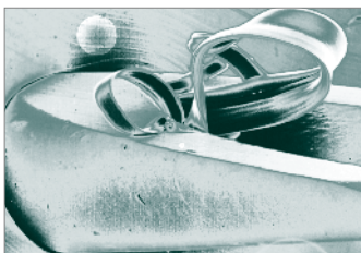
Coring of the silicone septum
